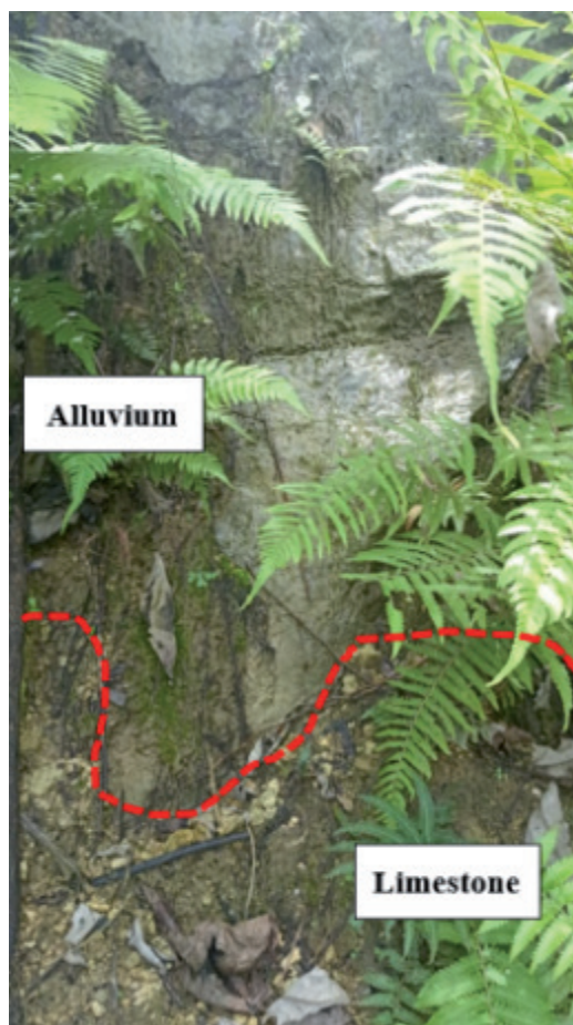
Figure 15. Rock layers on the cliff wall at Line 4 at the 15 meter point in the direction of the track: limestone begins to be visible at a depth of 2.5 meters.
