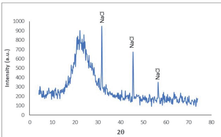
Figure 3. XRD Pattern of as-received silica from hydrothermal site
